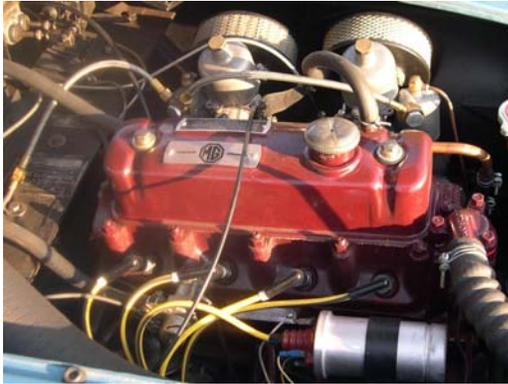
Before starting, you might want to take a compression test of your engine for which you will need a compression gauge. To start, remove the spark plugs, disarm the ignition system, install the compression gauge in each of the cylinders, one at a time and rotate the engine with the starter about six revolutions for each cylinder tested and take note of the readings. If they are fairly equal, you do not have a big problem. GOOD.
