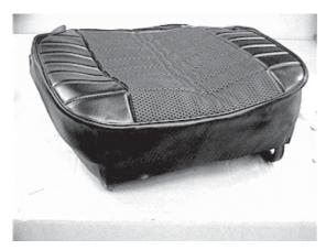
Slits must then be made in the vinyl material, approximately one inch long, where the forward frame tubes come down. This is necessary to allow the material to "clear" these pipes.
