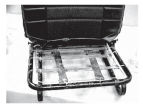
Temporarily bolt the seat frame back & bottom back together. This must be done to properly align the upholstery flutes of the back & bottom upholstery.
