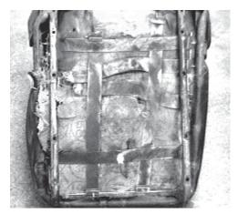
The headrest must be removed first, to allow proper access for upholstery removal. It simply pulls (with some difficulty) straight up, and out of the seat back. Don't be scared to apply a little muscle.
