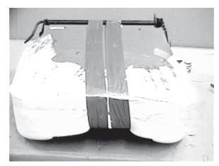
Plastic strip glued around the periphery of the seat.
