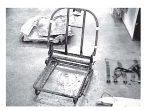
If the seat frame is severely rusted, we recommend replacing it with a better one. Keep in mind that there is a lot of force exerted on the seat during hard acceleration! It would be extremely disappointing to go through the expense and labour of seat rebuilding only to have the frame break!
