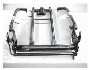
Here is the seat back frame with new back foam installed. It is simply glued in place with contact cement.
