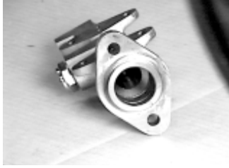
Empty cylinder-ready for inspection.
