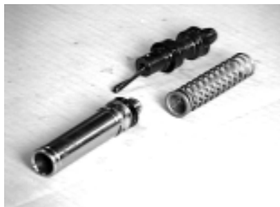
Everything separated – ready for seal replacement.
